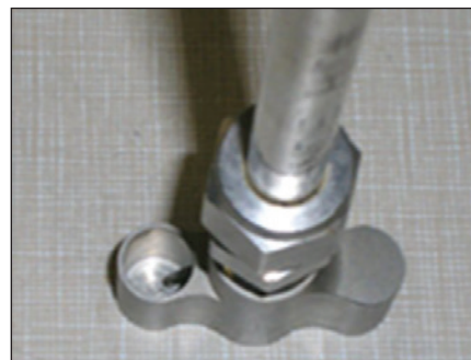
Figure 2. Reusable probe tip.
