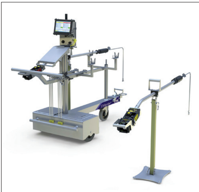
Figure 1. STARprobe kit with mobile station and monitoring system (left) and portable stand showing the probe tip, lance, and head ready for measurement (right). 3
